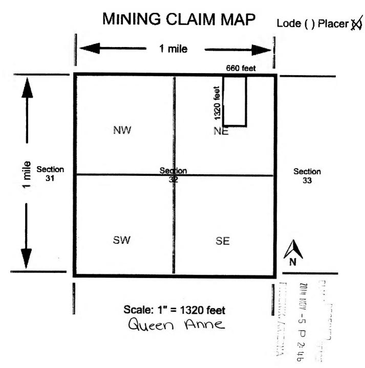
The NW corner of the claim is 3960 feet in a East direction from a survey monument described as the NW corner of Section 32, Township 25 North, Range 8 East, Coconino County Arizona.
