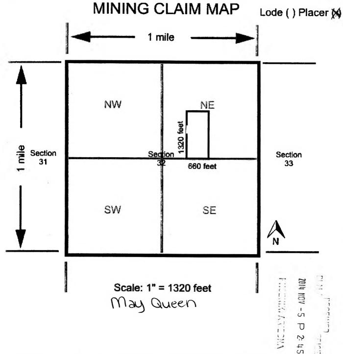
The NW corner of the claim is 3300 feet in a East direction, then 1320 feet in a South direction from a survey monument described as the NW corner of Section 32, Township 25 North, Range 8 East, Coconino County Arizona.
