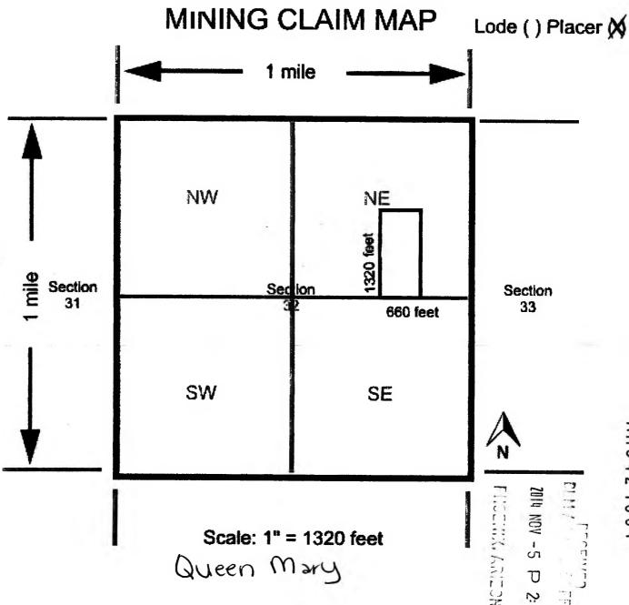
The NW corner of the claim is 3960 feet in a East direction, then 1320 feet in a South direction from a survey monument described as the NW corner of Section 32, Township 25 North, Range 8 East, Coconino County Arizona.
