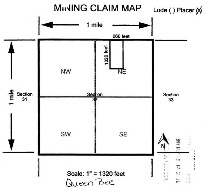
The NW corner of the claim is 3300 feet in a East direction from a survey monument described as the NW corner of Section 32, Township 25 North, Range 8 East, Coconino County Arizona.
